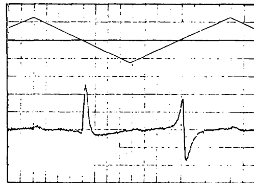
Fig. 4: Transmitted light, triangle-wave modulation. Total time is 50mS, slope is 40gs/sec.
